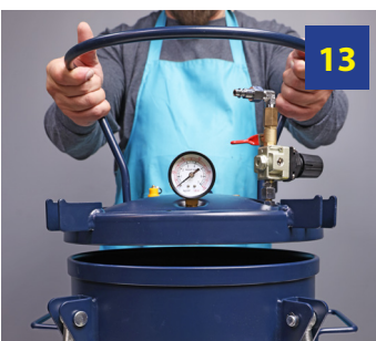
13 Carefully loosen wingnuts & gently lower the holding bolt fixtures to remove lid.
