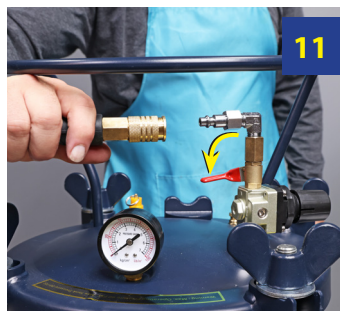
11 Close air control valve and disconnect the air supply.
