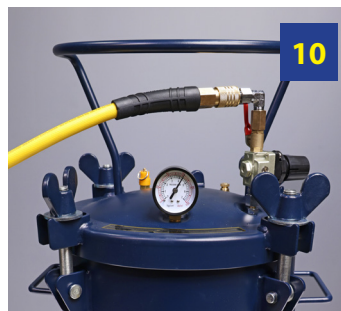
10 Keep the air supply connected until material in mold fully cures.
