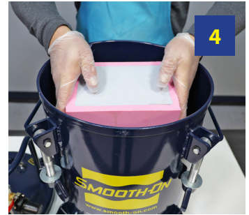
4 Place a resin-filled mold inside the pressure chamber.
