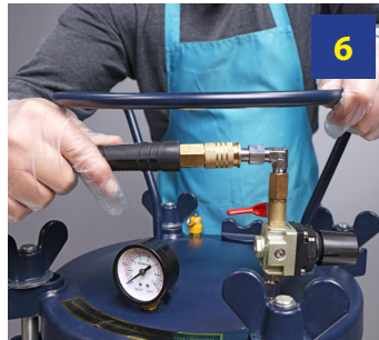
6 Using the quick connect fitting, attach an air supply hose.
