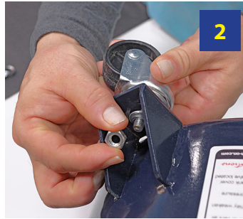
2 Use nut & washer to attach the 4 wheel assemblies and secure with wrench.
