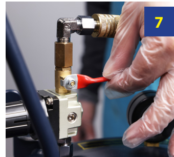
7 Make sure the air compressor is on and fully charged. Initiate the air flow into the pressure chamber by lifting the air control valve lever.
