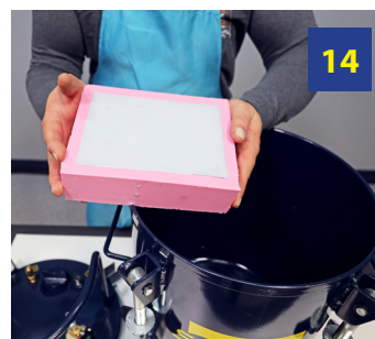
14 Remove rubber mold and cured casting from chamber.
