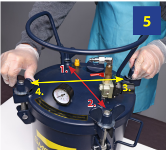
5 Align and secure the lid by tightening the wing nuts two at a time, opposite each other.
