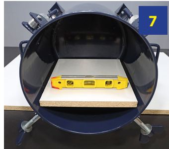
7 Place a board to use as a level surface inside the pressure chamber.
